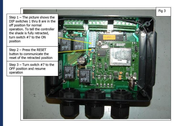
4) There is no need to reset the extended position once the correct HOME position is reset. Because the home position is now set at the correct position, the system knows exactly how far to extend. Adjustment is now complete.
