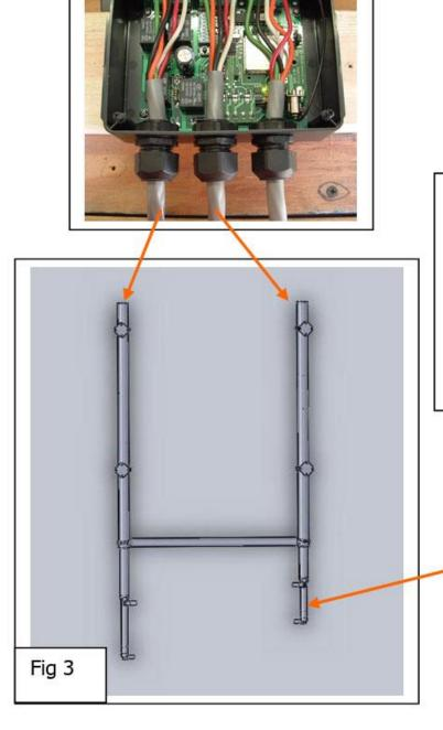
If the middle control cable is connected to the starboard actuator as shown in Fig 3, then turn switch #5 to the ON position and extend the actuator to be in alignment with the port actuator. Then turn switch #5 to the OFF position.
